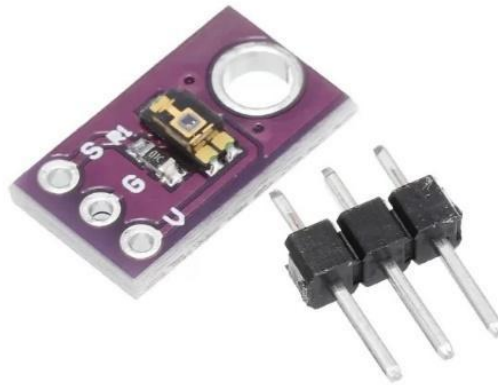
SEQ figure \* ARABIC 4. Fig. Analog luminance sensor Image source: https://www.microcontroller.hu/termek/temt6000-fenyerosseg-mero-szenzor/
