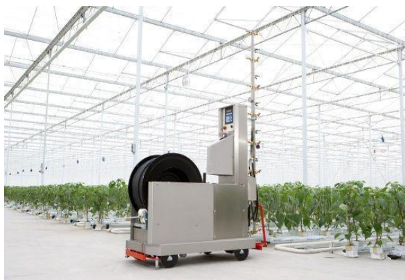
Self-propelled, greenhouse spraying robot and spraying wheel for ultra-low rates of plant protection products
